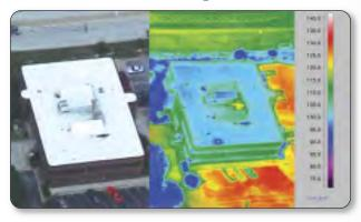
On hot summer days, the temperature on dark surfaces – including asphalt parking lots and roofs – can reach 180 degrees or higher, straining HVAC units and increasing energy use. The highly-reflective Duro-Last Cool Zone membrane can dramatically reduce roof surface temperatures, lowering cooling costs and keeping non-conditioned space more comfortable and productive for workers. A Cool Zone roof also helps lessen the urban heat island effect.
